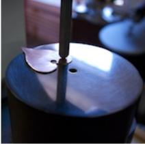
The next photo shows me putting pressure on the stamp by rotating the arbor press shaft with my right hand while I strike the arbor (once) with a hammer.
